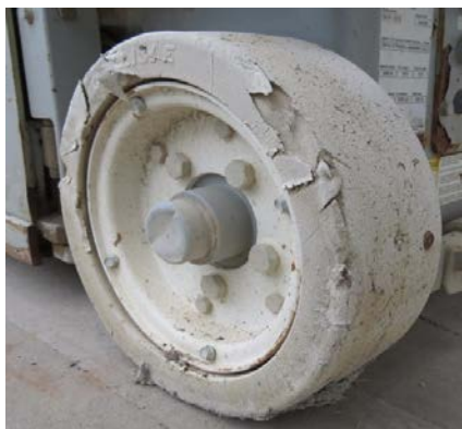
Excessive damage to sidewall and separation between tyre and rim
