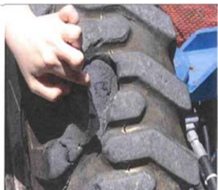
UNACCEPTABLE – Sever tread damage complete lug can be peeled away
