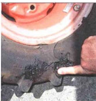
UNACCEPTABLE – Severe side wall damage
