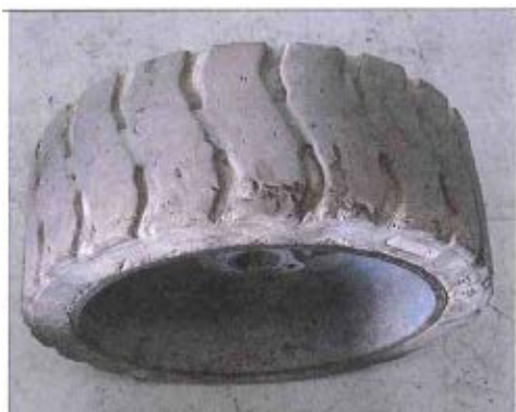
Non Critical – Small amount of tread damage and minor wear
