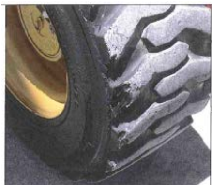
Non Critical – Small amount of tread missing
