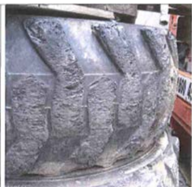
UNACCEPTABLE – Severe tread wear
