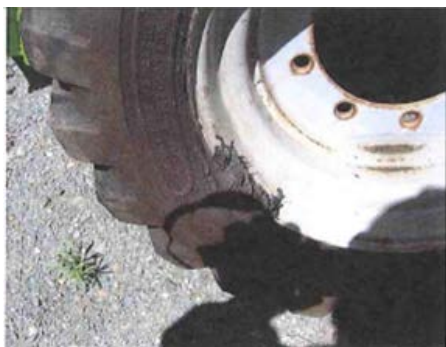
UNACCEPTABLE – Bead damage
