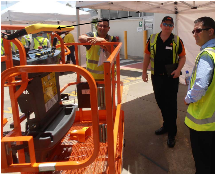
Figure 2 Pressure Sensing Device (Arrowed)
