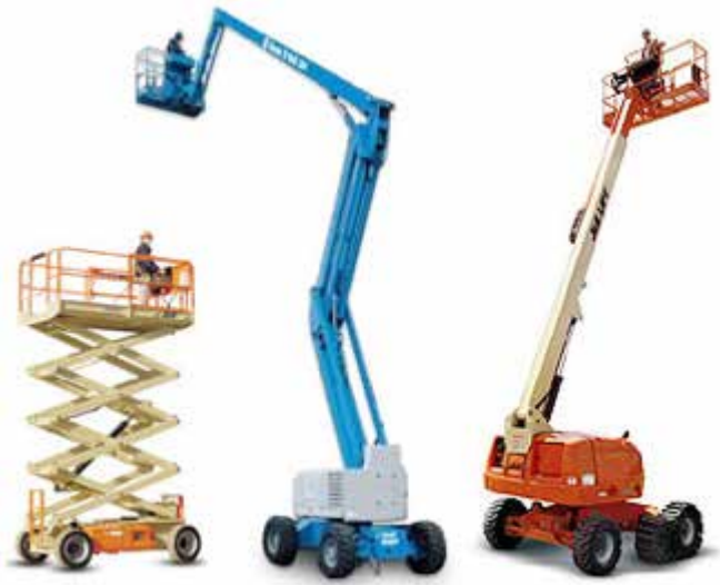
Above: three types of Elevating Work Platform – a scissor lift, an articulating boom lift and a straight boom lift
