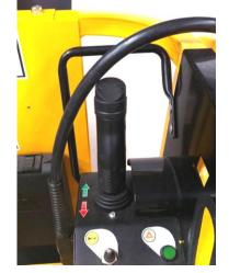
NOTE: WELD HOSE FORCED INTO POSITION – WILL NOT SLIDE AROUND JOYSTICK WITHOUT OPERATOR MANIPULATION
