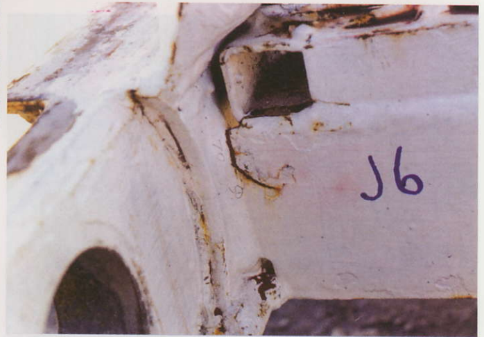
Above from left to right: Magnetic testing on a dockside crane with an electromagnet and squeeze ball of magnetic particles; Rust helps locate possible crack locations - but only further testing can confirm their existence
