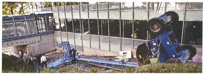
Lesson Learned Summary: A double fatality occurred when a man lift toppled over at a construction site. The two men were operating a Genie S85 telescopic boom on uneven ground and had incorrectly positioned the Lift's counter weight on the downhill side of the slope.
