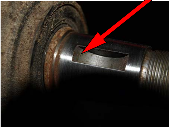
Use die penetrant to check for cracks in the key way area.
