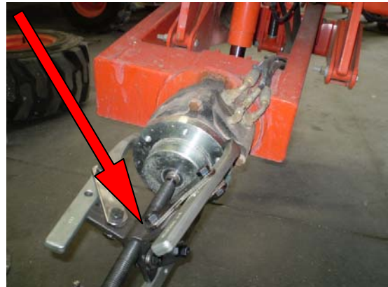
Use a puller or suitable pulling equipment to Remove hub from stub axle.
