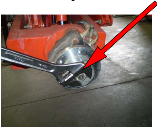
Remove nut holding hub to stub axles
