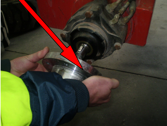
Use die penetrant to check for cracks in the key way area.
