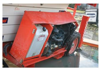
The parts of the machine that have some value and are useable are: Deck and handrails Hydraulic Manifolds Lower control box Engine Stabiliser cylinders (2)
