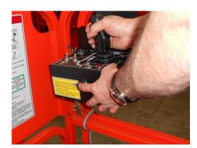
3. Release Enable Switch. Operate as normal
