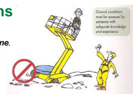
If ground conditions are poor, do not operate the MEWP.
