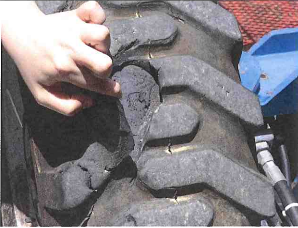
UNACCEPTABLE - Severe tread damage – complete lug can be peeled away
