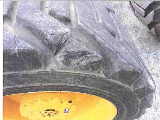
Non-critical - Small amount of tread missing but outer case is not damaged.
