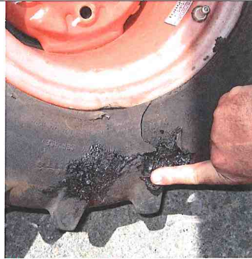
UNACCEPTABLE – Severe side wall damage
