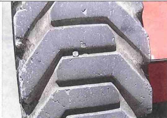
Bolt in tyre –this is not a fault - bolt is used to plug the air hole after filling.
