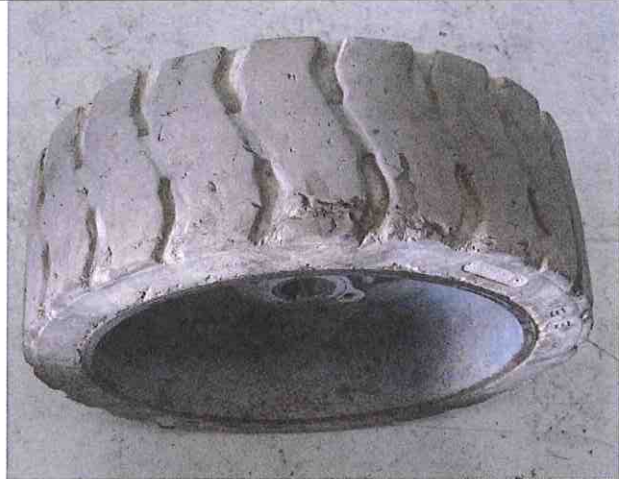
Non-critical - Small amount of tread damage and minor wear
