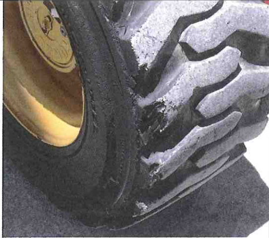
Non-critical - Small amount of tread missing
