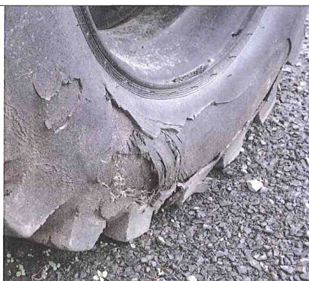
UNACCEPTABLE - Severe side wall damage – foam filled tyre
