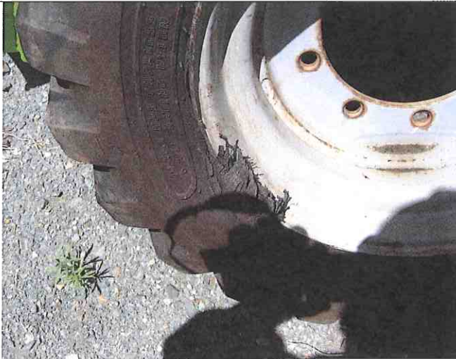
UNACCEPTABLE - Bead damage.
